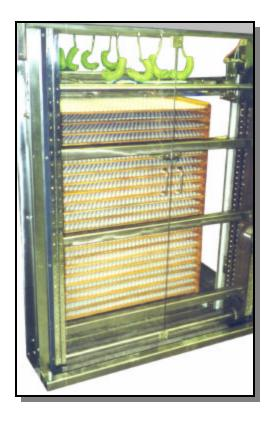
This custom tray stacker was designed to be integrated into an existing production line for handling 19.5-inch X 37-inch wooden trays filled with product.
