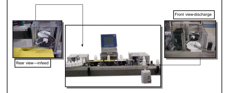
Wrabacon's Rotary Transfer System was designed to take small plastic bottles out of the conveyor line, feed through a checkweigher on 9 inch centers, and discharge back onto the same conveyor.
