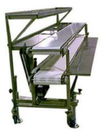
*Wrabacon* designed and manufactured two of these stainless steel, wash-down capable conveyors for a company that packages frozen chicken products.
