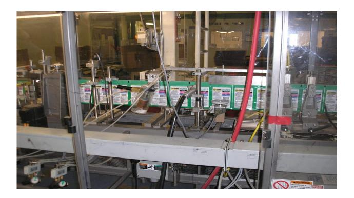
Wrabacon designed the mechanical mounting and software for a vision system to inspect and verify date code, bar code and OCR of the bar code on individual bags for this high speed vertical bagger. The bags passed the vision system at the rate of 110 bags per minute. The bags are 4 ¾ inch wide x 8 inches long and were printed via ink jet prior to the vision system. Wrabacon provided all mechanical set up, vision system and software, along with a system control panel.
