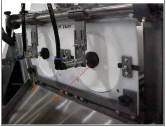
Step 3: Immediately upon connection, the overhead conveyor seals the lid onto the container. Lids and containers are kept under constant control at all times.
