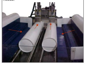
**Step 2:** The dual pick heads alternate denesting the lids from the horizontal stacks and place them into the chute.
