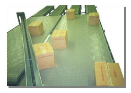
This particular Wrabacon servo merge conveyor will accept incoming product in four rows. This system does not require any form of gate and release system. Product is not stopped prior to entering the servo merge. The system will also accept product in a random manner.
