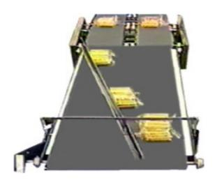
Wrabacon's servo merge does not require any form of gate and release system. Product is not stopped prior to entering the servo merge. The system will also accept product in a random manner. The servo merge system consists of a gap, correction, and merges conveyor sections. The system functions in the following manner:
