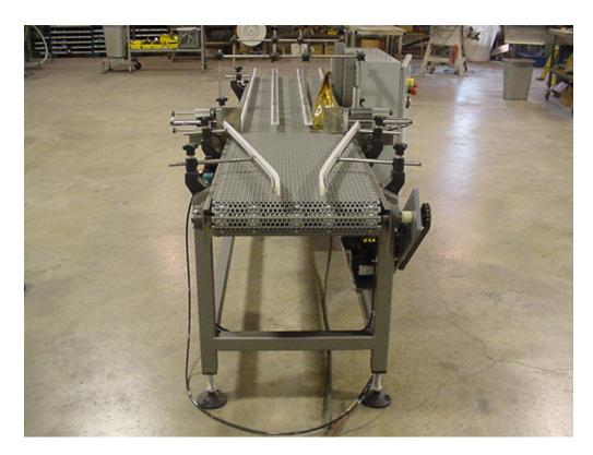
Wrabacon custom designed this 2-1 gate and release merge to merge stand up pouches of premium chocolate. The system was designed to merge pouches at the rate of 50 pouches per lane. The Allen Bradley PLC was programmed to provide the system the ability to merge several different size pouches. This merge was integrated into the customers' new pouch filling line.
