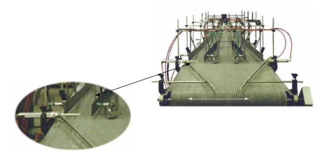
This unique Merge Conveyor is part of a Product Handling System designed and manufactured for a cookie baking company that was looking for ways to improve product-per-package-count accuracy and increase overall product output. This 3-lane conveyor has LED displays that accept data from a serial output from an upstream checkweigher, and multiple photo sensors that operate timed stop and release gates (shown in outset) to aid operators and control flow at the downstream end of the conveyor.
