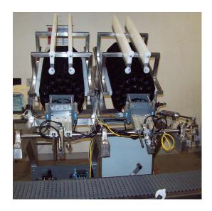
Wrabacon's twin magazine tray denester is designed for easy change over for different size trays. System is designed to be added to an existing packaging line. Rates vary depending on size and weight of trays. Typical rates are in the range of 17-20 trays per magazine. As with all Wrabacon equipment these tray denesters can be manufactured in stainless steel or mild steel.
