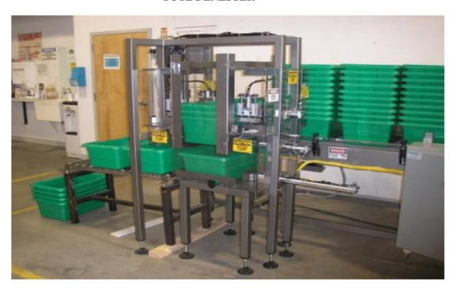
Wrabacon custom designed this tote denester to denest plastic totes at a rate of 2 per minute. The totes measured 12 inches wide x 21 inches long and weighed 3.25 lbs. The system was designed to have in queue 40 totes in stacks of 10 high. Equipment supplied within the system included a 36 inch long split belt conveyor, denester, accumulation conveyor, auto load into the denester and full control system.
