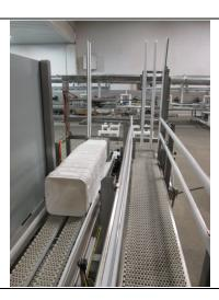
Wrabacon's pail denester is designed to accept stacks of pails which are transferred to a tip down device that lays the pails down on their side. Once on their side pails are transferred to a mechanism that pulls the pail from the stack and turns them up right to be transferred to downstream filling equipment.
