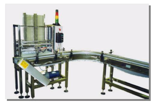
This *Wrabacon* Automatic Container Denester System with accompanying conveyor was designed and manufactured to cut production losses for a company using a thermoformer in its manufacture of plastic trays. Prior to the *Wrabacon* system, when the thermoformer was down, the entire production line was down. The *Wrabacon* system was designed to fit between the thermoformer and the remainder of the down-stream system to provide continuous production capability.
