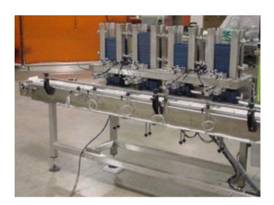
Wrabacon custom designed this tray denester to denest trays at the rate of 100 trays per minute. The System was designed to denest trays on an indexing conveyor which then transported the trays to an overhead filling system. Once filled, the trays were conveyed to the packaging area for further process.
