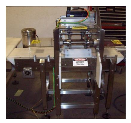
This servo controlled overhead reject sweep is designed to reject product from either a check weigher, metal detector or X-ray inspection equipment. A signal is sent to rejector, once the article enters the system an overhead paddle sweeps the product into a reject bin. The system can be manufactured either stainless steel or painted steel.
