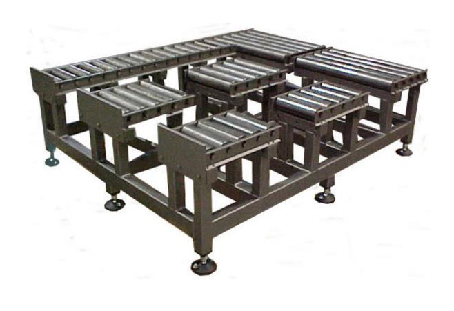
On this pallet roller conveyor, pallets roll down a slight decline before reaching a fixed stop. With 9 inch gaps between sections, forklift operators can access the pallets from two sides. This particular unit is built on one frame and consists of 6 sections. I has been constructed of heavy duty painted steel with adjustable (+/- 2") foot pads. The over-all dimensions are 64" long x 54" wide x 21"-22" high.
