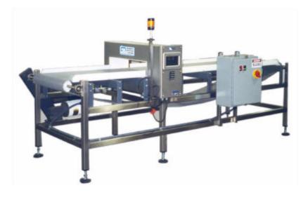
This custom Metal Detector Conveyor is the primary unit of a four-piece conveying system designed and manufactured for a large baking and distributing corporation. The Metal Detector Conveyor is 10 feet long, 24 inches wide and the frame is of stainless steel construction. The conveyor belt is durable, long-lasting Polypropylene.
