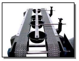
*Wrabacon* designs and manufactures custom conveyors for all types of labeling applications, including bottom, top and side labeling. While this particular design was for a bottom, pressure-sensitive labeler, we have also designed and manufactured conveyors for print and apply, ink jet, and laser coding systems.
