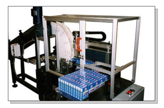
Case packing is the focus of this custom made Product Collator. A well known dry-soap supplier needed to orient soap detergent boxes into rows of 11 in order to help their operators load them into cases more efficiently. Wrabacon accomplished this with this simple and cost effective design.
