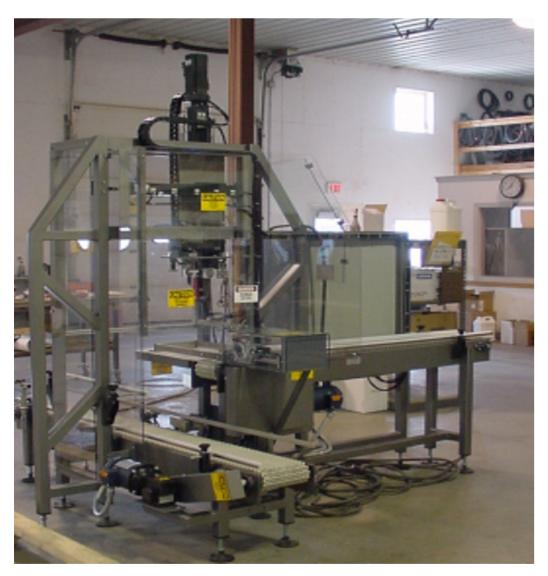
Wrabacon custom designed this 2.5 plastic bottle case packer to case pack at a rate of 18 containers per minute. Containers measured 8.5" x 7" long x 18" high and weighed 18 lbs. Containers were received single file and were pushed 90 degrees into the pick area. Once two containers were located in the pick area a pick and place module picked the two containers placed them into an erected carton that was located on the bottom conveyor.
