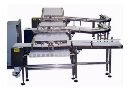
This System represents one of *Wrabacon*'s more extensive design successes in developing, programming and manufacturing multiple, interacting components for a food processing corporation. The system accepts trayed product from one of three productions lines, orients and transfers product to a freezer infeed conveyor, then receives product from the freezer, places them in the required orientation and conveys them downstream.
