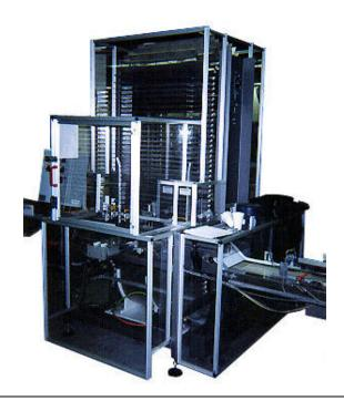
Wrabacon's Vertical Accumulators take up minimal floor space and they are a very reliable form of product accumulation during those unpredictable times of downstream equipment delays.
