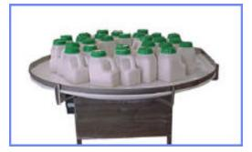
*Wrabacon's* rotary accumulation tables are designed to integrate with a customers' existing production lines at both infeed and discharge ends.
